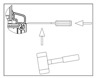
Carefully place a chisel as shown between the profile and glazing bead and knock out the latter with a rubber hammer.
